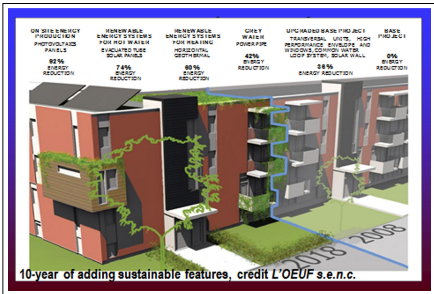
Figure 2. Stages of improvements from 2008 to 2018 in Atelier Rosemont, Montreal (credit: L'OEuf s.e.n.c (65)).
